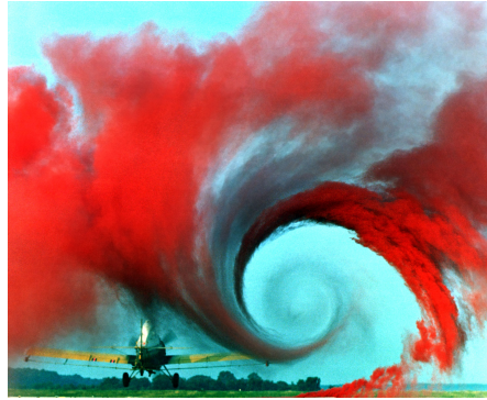
FIGURE 1.1: The air flow from the wing of an agricultural plane made visible by a technique that uses colored smoke rising from the ground. [75]
