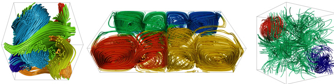
FIGURE 6.12: Streamline visualizations colored using spectral clustering of the flow domain. The datasets from left to right: ABC flow, Bénard flow, Borromean magnetic field.
