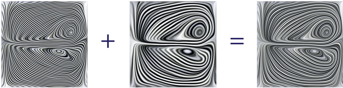
FIGURE 5.8: Two flow visualization images centered around different frequencies are averaged to obtain the image at the right. The result features the frequencies of both input images.
