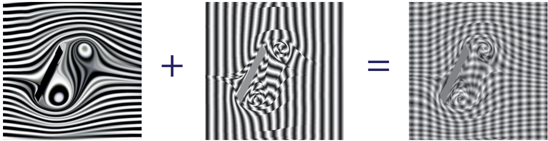
FIGURE 5.12: Left: OGR LIC image with period 12 pixels across the flow. Middle: OGR LIC image with period 24 pixels along the flow. Right: One animation frame, obtained by blending the first two images. The subsequent frames are computed by incrementing the phase of the image in the middle.
