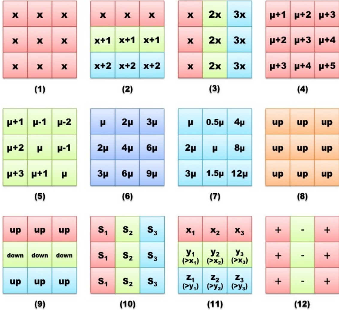
Figure 2.2: Demonstration of bicluster models. (1) Constant bicluster, (2) Constant rows, (3) Constant columns, (4) Coherent values with additive model, (5) Coherent values with additive model, (6) Coherent values with multiplicative model, (7) Coherent values with multiplicative model, (8) Coherent evolution with constant up-regulation, (9) Coherent evolution with constant up-regulation and down-regulation arranged by rows, (10) Coherent evolution with constant status arranged by columns, (11) Coherent evolution with preserved order, (12) Coherent evolution with preserved (positive/negative) changes.
