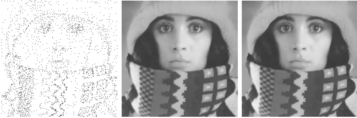
Figure 4.8. Tonal optimisation for EED inpainting. Left: Prescribed inpainting mask (density: 4%). Centre: EED inpainting with tonal values from original image trui (MSE: 12.62). Parameters: \lambda = 0.8 , \sigma = 0.7 . Right: Inpainting with optimised grey values (MSE: 10.79).
