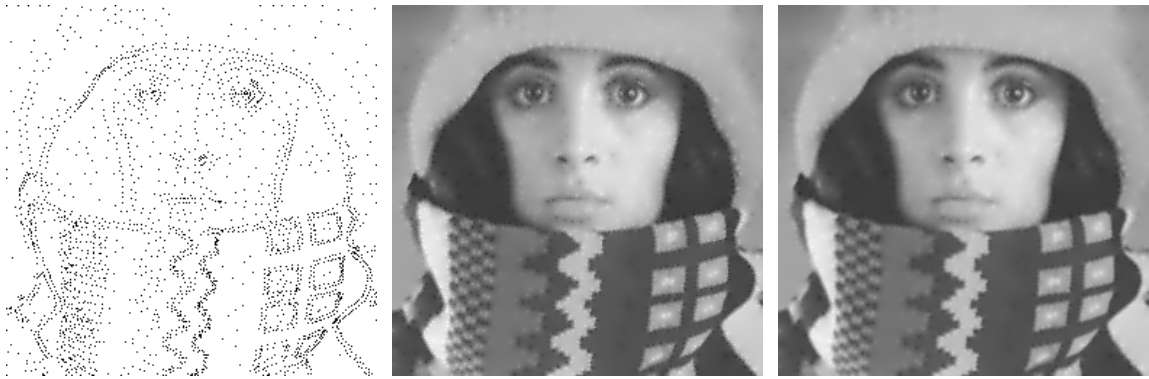
Figure 5.10. Spatial optimisation for homogeneous diffusion inpainting with gradient descent using discrete Green’s functions and a mask density of 4%. Left: Final mask with points at grid locations. Centre: Corresponding tonal optimised inpainting (MSE: 25.6). Right: Optimised inpainting with continuous mask locations (MSE: 16.81).
