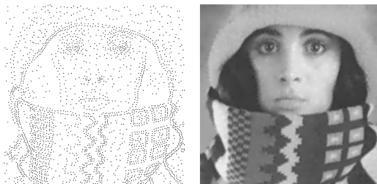
Figure 5.7. Spatial optimisation for harmonic inpainting with improved analytic approach. Left: Optimised mask (density: 4%) with Algorithm 5.5 (parameters: \sigma = 1.0 , p = 0.98 , \tau = 1.55 , q = 2.51 ). Right: Corresponding tonal optimised inpainting (MSE: 25.71).
