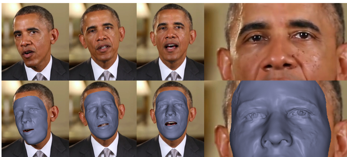
Figure 7.1: Result obtained by the proposed approach on a video downloaded from YouTube. Top: Input video ( https://youtu.be/d-VaUaTF3_k ). Bottom: Reconstructed high-quality, personalized 3D model that captures: Coarse-scale face geometry and expressions, medium-scale person-specific idiosyncrasies, and fine-scale skin detail – all directly from monocular video.
