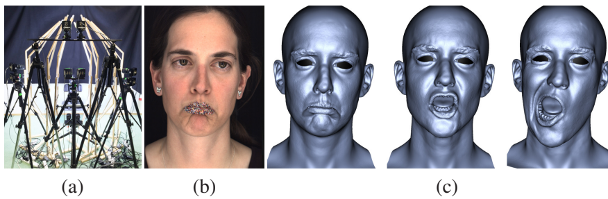
Figure 9.3: High-quality lip database. Using a controlled multiview capture setup (a), and lip tattoos (b), high-quality lip shapes are reconstructed for training (c).
