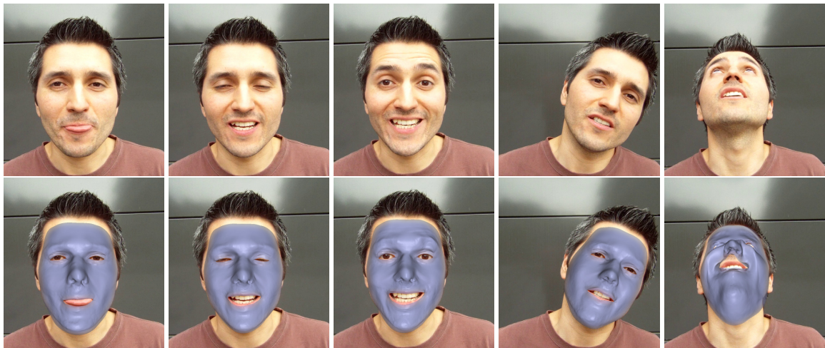
Figure 5.10: Results captured with a hand-held GoPro camera - fourth sequence, 650 frames (22 s). This sequence was recorded outdoors under unknown lighting and features challenging head motion. The rightmost column shows a failure case where our method does not estimate the pose and expression correctly. The supplementary video at the project website shows that our method fully recovers afterwards.
