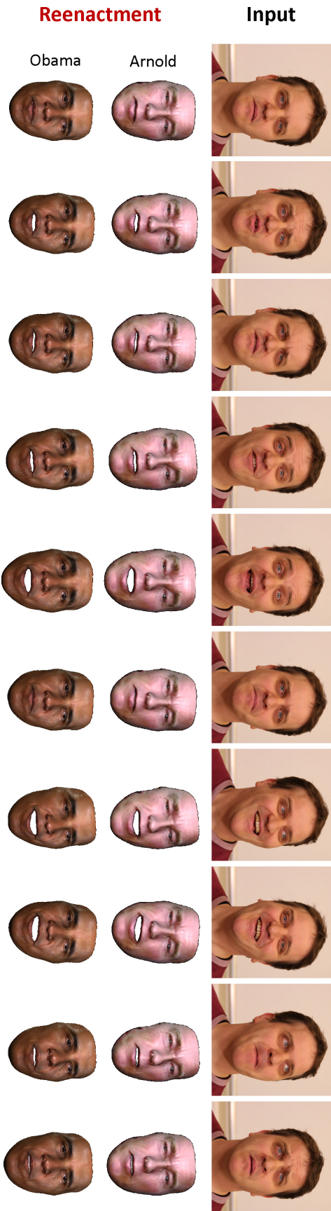
Figure 8.7: Facial reenactment. Here, we retarget the rigid head pose and the non-rigid facial motion (coarse expressions) of SUBJECT2 (top row) to the high-quality 3D rigs of two target actors: ARNOLD OLD (middle row) and OBAMA (bottom row). Since the detail layers are regressed for every input expression, the target actor's characteristics are effectively preserved in the reenactment.
