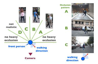
Figure 4.4: Bird's eye view of occluded person's state space (*left*). Synthetically generated training images for different occlusion patterns and walking directions (*right*).
