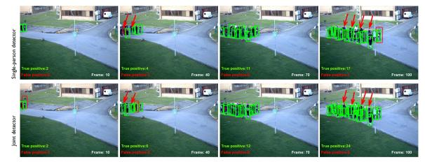
Figure 4.9: Detection results on the PETS S1.L2 dataset at precision 0.9 obtained with our DPM single-person detector (top) and our joint detector (bottom). The true positive detections are visualized using green and the false positive detections using red color. The red arrows indicate the detections mentioned in the text.
