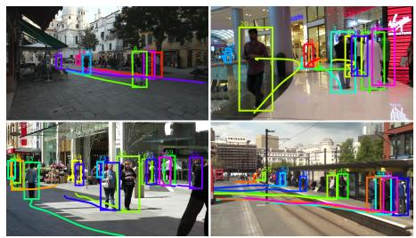
Figure 7.1: Qualitative results on the MOT16 Benchmark. The solid line under each bounding box indicates the life time of the track. The lifted multicut tracking model is able to link people through occlusions and produces persistent long-lived tracks
