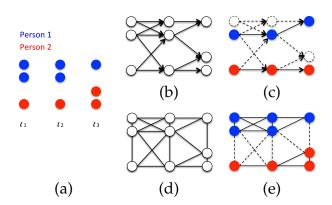
Figure 5.2: Two person detection hypotheses in three consecutive frames (ground truth assignment depicted in color) (a); The disjoint paths (c) obtained by solving a Minimum Cost Disjoint Paths Problem with respect to a directed graph (b); The decomposition (e) obtained by solving a Minimum Cost Subgraph Multicut Problem with respect to an undirected graph (d).
