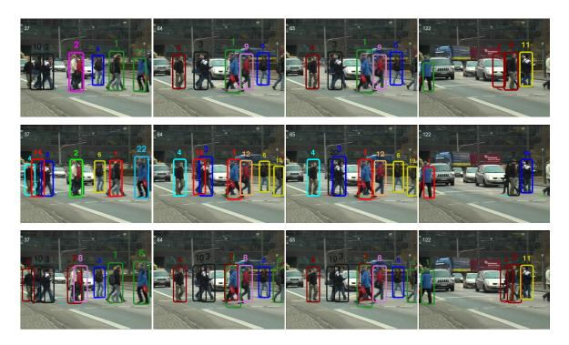
Figure 3.11: Tracking results on the TUD-Crossing dataset obtained with the approach of Andriyenko and Schindler, 2011 (top row), our single-person detector (middle row) and our joint detector (bottom row). Colors and numbers indicate tracks corresponding to different people.
