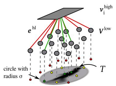
Figure 8.2: Edges  $e^{\text{hl}}$  between high and low level nodes. For every detection  $v_i^{\text{high}}$ , an edge with an attractive cost  $c_e^{\text{hl}}$  is introduced when it hits the according template *T* (green edges). If the template is not hit and the distance is larger than a threshold  $\sigma$  (indicated by the gray circle), an edge with repulsive edge cost is introduced (red). If the template is not hit but the distance is smaller than  $\sigma$ , no edge is introduced.
