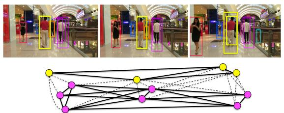
Figure 6.1: An example for tracking by multicut. A graph (bottom) is built based on the detections in three frames (top). The connected components that are obtained by solving the multicut problem indicate the number of tracks (there are two tracks, depicted in yellow and magenta respectively) as well as the membership of every detection.
