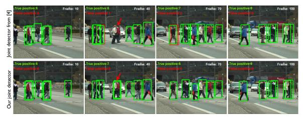
Figure 4.7: Detection results (every 30 frames) on the TUD-Crossing dataset at precision 0.95 obtained with the joint detector from Tang *et al.*, 2012 (top) and our joint detector (bottom). The true positive detections are visualized using green and the false positive detections using red color. The red arrows indicate the detections mentioned in the text.
