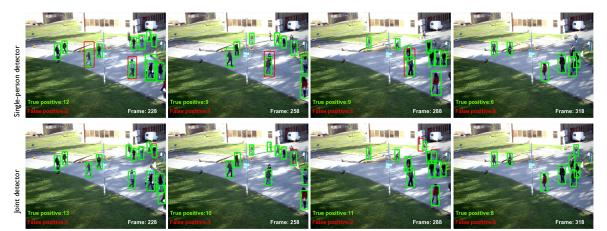
Figure 4.8: Detection results on the PETS S2.L2 (test sequence, frames 228–436) at precision 0.9 obtained with our DPM single-person detector (top) and our joint detector (bottom). The true positive detections are visualized using green and the false positive detections using red color. The red arrows indicate the detections mentioned in the text.
