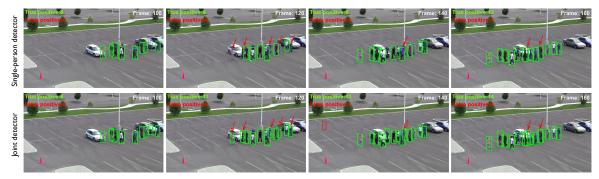
Figure 4.10: Detection results on the ParkingLot dataset at precision 0.95 obtained with our DPM single-person detector (top) and our joint detector (bottom). The true positive detections are visualized using green and the false positive detections using red color. The red arrows indicate the detections mentioned in the text.
