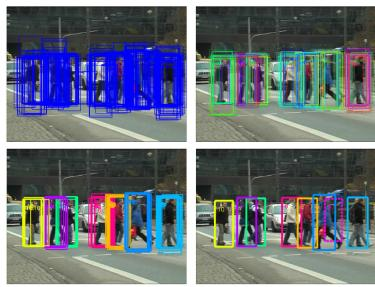
Figure 5.1: Overview of the Subgraph Multicut tracking method: (clockwise) detection hypotheses, overlapping tracklet hypotheses, hypotheses decomposition (clustering jointly across space and time) and final tracks (dotted rectangles are interpolated tracks).
