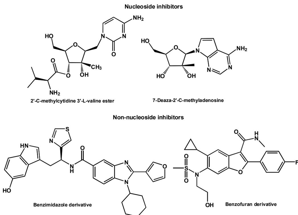
**Figure 8:** Structures of potential NS5B inhibitors.
