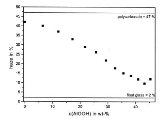
Fig. 3. Abrasive resistance (% haze) [5] in dependence on AlOOH concentration compared to floatglass (haze = 2%) and polycarbonate (haze = 47%). Coated substrate: PC, UV hardened, coating thickness: 5  $\mu$ m.
