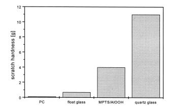
Fig. 4. Scratch hardness of different substrate materials (PC, float glass, quartz glass) compared with the matrix system of 43.2 wt.% AlOOH on PC, coating thickness: 5  $\mu$ m.
