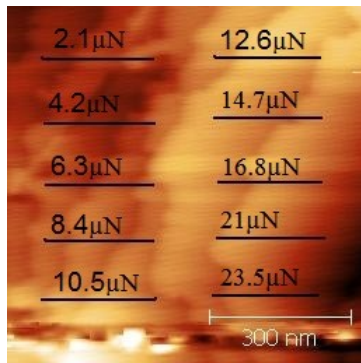
(a) Image of the scan area where the ten line scratches of different loads were proposed.
