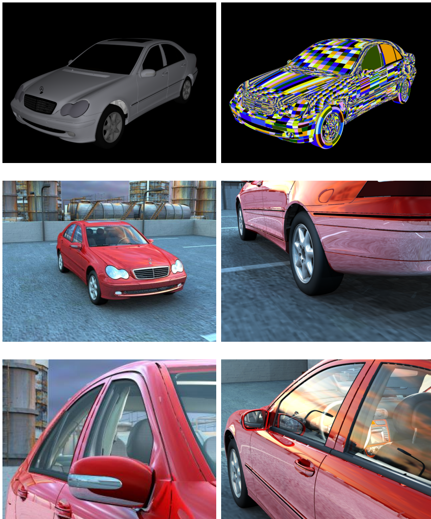
Figure 6.23: Top left: Mercedes C-class model directly exported from a CAD system and converted into 319,340 bicubic Bézier patches and 1.46 million (bicubic Bézier) trimming curves. The patches are ray traced directly without triangulation. Top right: In order to illustrate the complexity of the Mercedes model, a random color is assigned to each patch. Center left: The model with advanced shading for glass and car paint, combined with surrounding geometry and an HDR environment map. Center right, Bottom left, Bottom right: Close-ups demonstrating the high geometric accuracy necessary for high-quality visualization of smooth surfaces.
