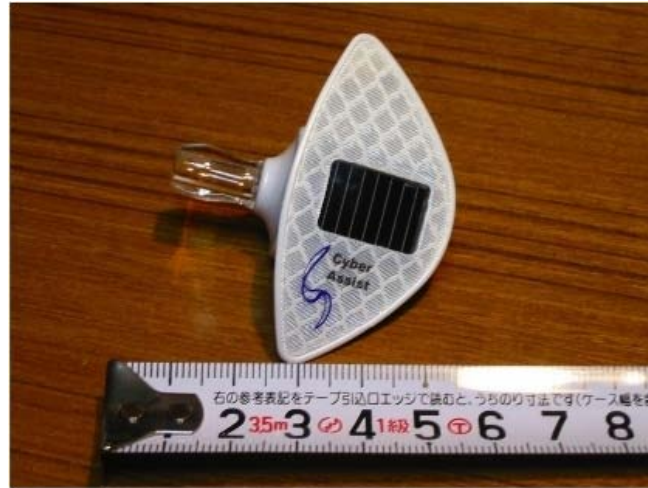
Figure 3.4: CyberAssist - devices for unified access to location based services (adapted from [Nishimura et al., 2002]).
