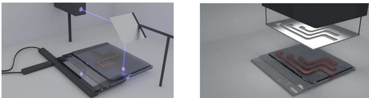
**Figure 40:** Schemes of techniques that can be implemented with different light sources **A.** direct laser writing **B.** photolithography.
