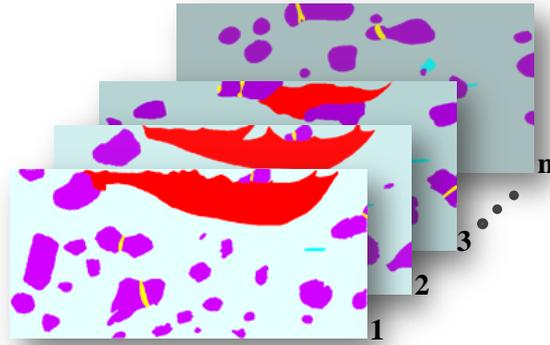
Figure 3.3: A bunch of labeled SEM images. Each phase is given a different color: Si particles are in magenta, intermetallic phases are in cyan, cracks are in yellow and a large pore is in red, aluminium matrix is transparent. The 3D volume is reconstructed by interpolation of the labeled features given a voxel size.
