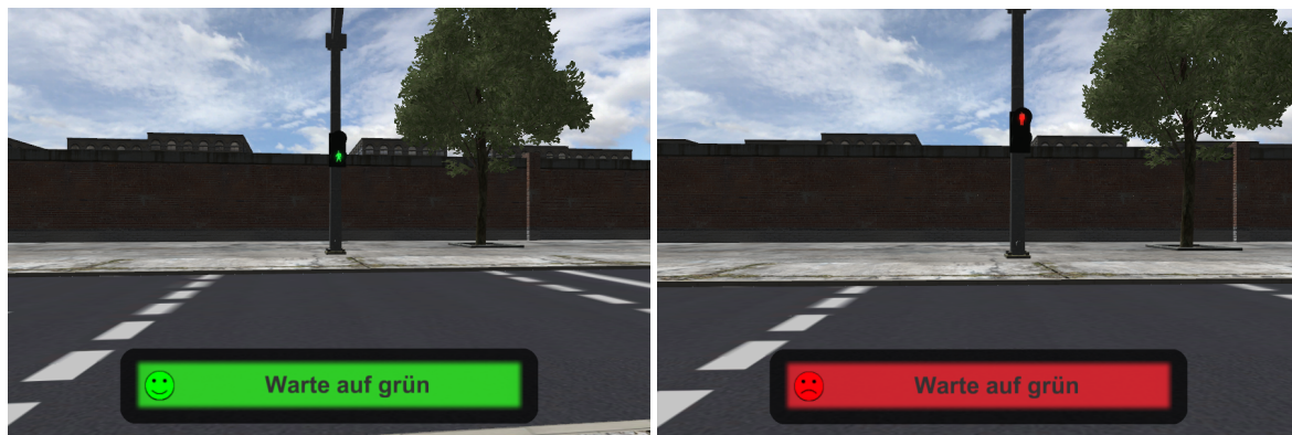
Figure 5.18: Immediate feedback. The instructions shown in Figure 5.17 transforms to the left image when the user has correctly waited for the light to turn green and to the right one if s/he failed to do so and entered the road prematurely.
