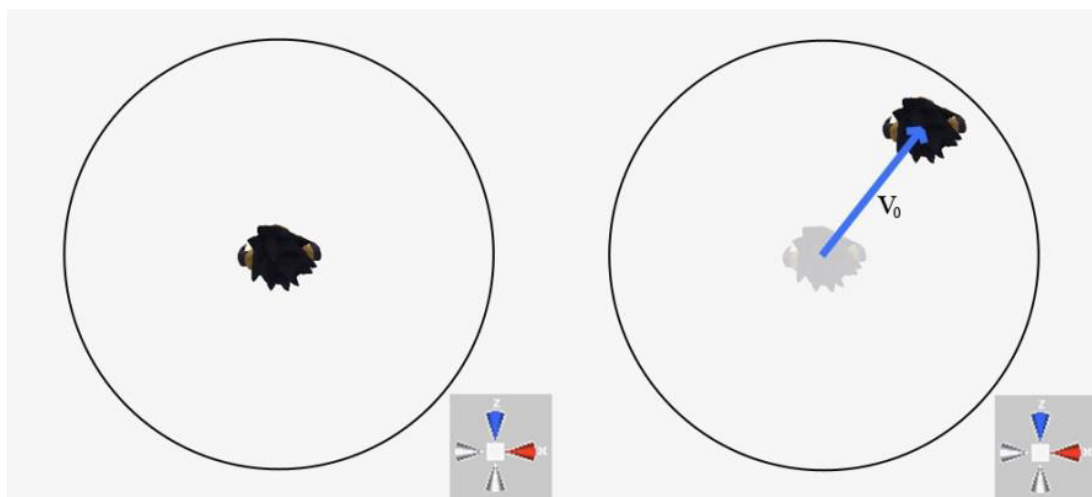
Figure 5.10: Distance-To-Velocity gesture for translational movement (Rump, 2014)
