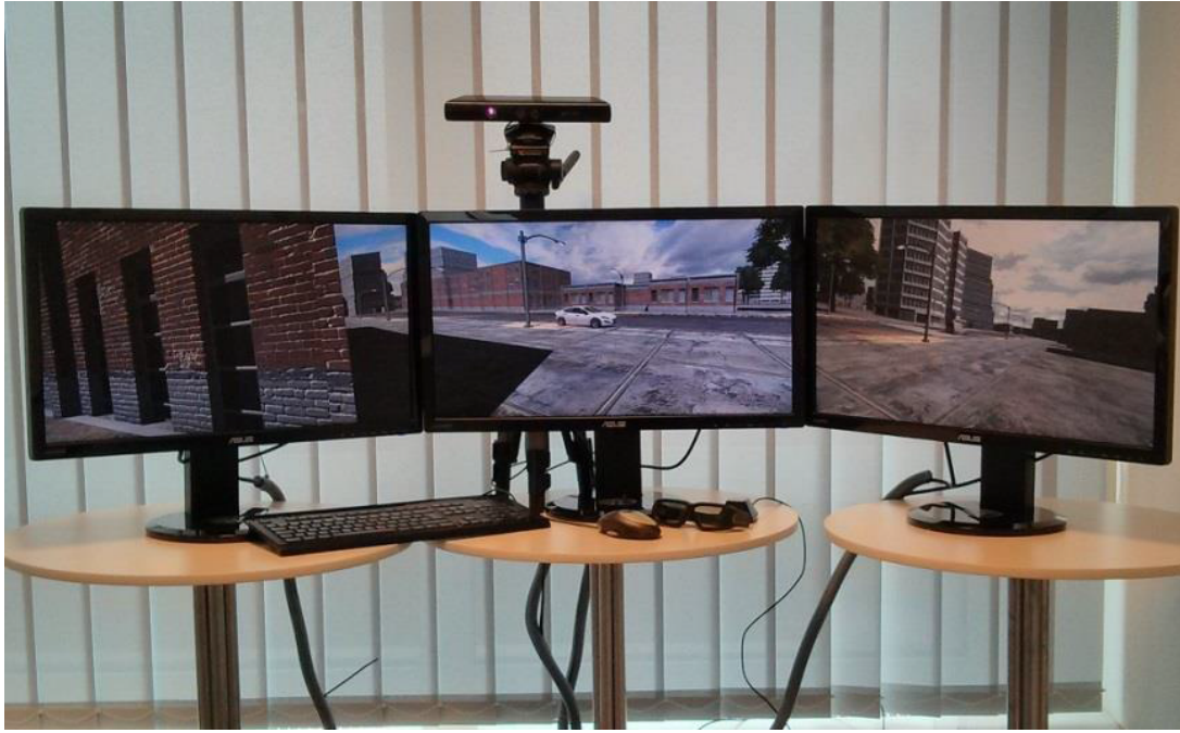
Figure 5.5: Semi-immersive interaction setup of SafeChild (consisting of three active stereoscopic monitors and a Microsoft Kinect motion sensor)
