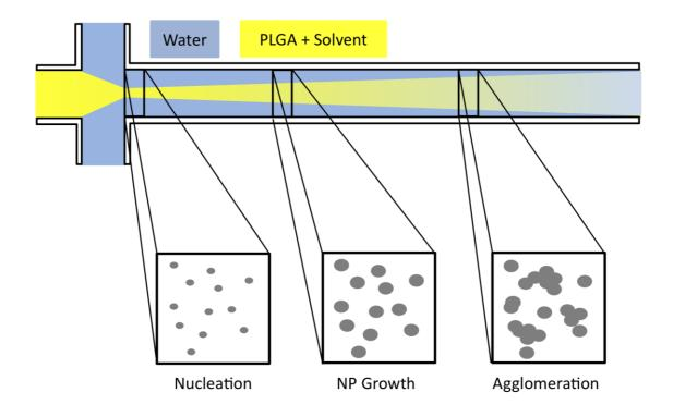
**Sketch 3:** Illustration of nucleation and growth mechanism of nanoprecipitation along the focus mixing channel in microfluidic system.
