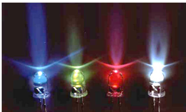
Figure 13. Blue LED and three LUCOLEDs emitting green, red, and white light. Reprinted with permission from Schlotter, P., Schmidt, R. & Schneider, J., Appl. Phys. A Mater. Sci. Process. A 64, 417–418 (1997). Copyright ©1997 Springer. 12
