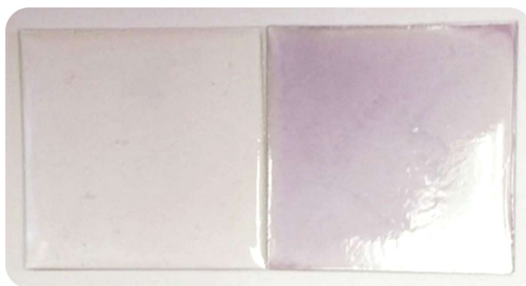
Figure 9. Consolidated coatings of melting gels on glass: (left) undoped and (right) with 2 ml of 10 nM Au-nanospheres solution added during the purification step. Gel composition is 65 mol% Methyltriethoxysilane –35 mol% Dimethyldiethoxysilane. Reprinted with permission from Klein, L. C. et al., J. Sol-Gel Sci. Technol. 89, 66–77 (2018), Copyright ©2018 Springer. 102
