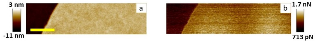
Figure 3.3: The topography (panel a) and adhesion (panel b) image of Polystyrene layer on top of a Polymethylmethacrylat layer, captured ex situ at room temperature, by Peak Force Microscopy mode. The thickness of PS is 14 nm. Scale bar presents 1\mu\text{m} on the sample.
