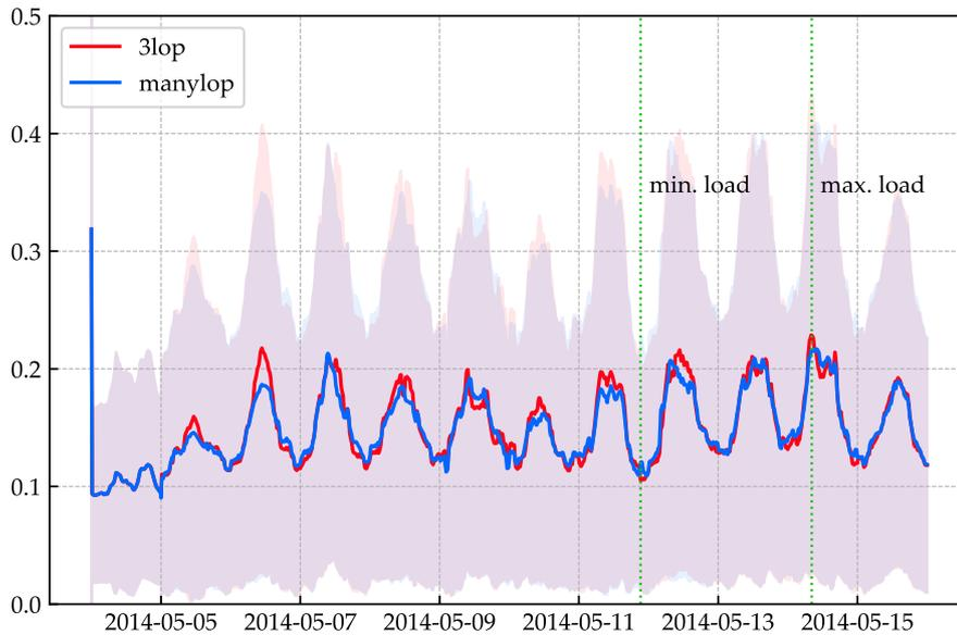
Figure 75: Details about the network load in the scenarios 3Lop and ManyLop: Usage rate of the individual lines over time. The red and blue lines show the average values of all lines per time slice in the two scenarios 3Lop and ManyLop respectively. The distributions of the utilization rate of all lines is indicated by the lower and upper boundary of the standard deviation given in light red and blue respectively. Cf. Figure 76.
