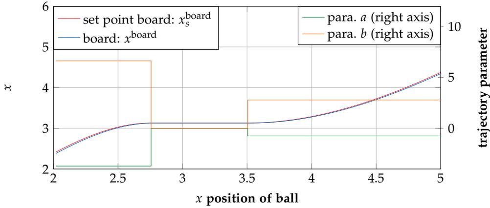
Figure 38: Behavior of the board ( $x^{\text{board}}$ ) in relation to the given trajectory ( $x_s^{\text{board}}$ ) and its parameters  $a$ ,  $b$ .
