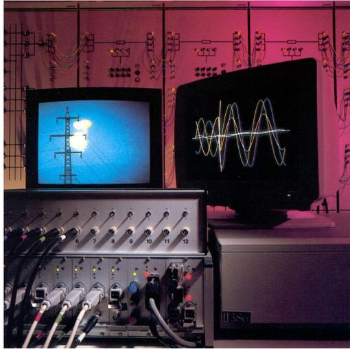
Figure 1: Photograph of a physical grid model (in the background) and measurement equipment (in the foreground) as used during the 90s at the Chair of Energy Supply at Saarland University.[15]
