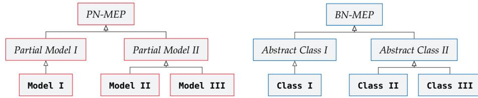
Figure 42: Parallel class structure of the MODELICA models and the C++ classes used by MOCES. *PN-MEP* and *BN-MEP* are abbreviations for *Physical Node - Mocses Entity Partial* and *Business Node - Mocses Entity Partial* respectively.
