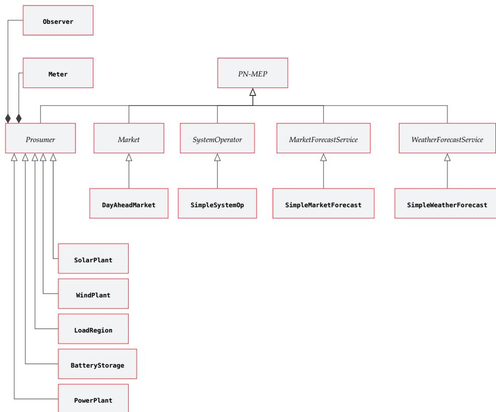
Figure 48: Base MODELICA models provide by MOCES to model the *Physical Node* part of a MENT.
