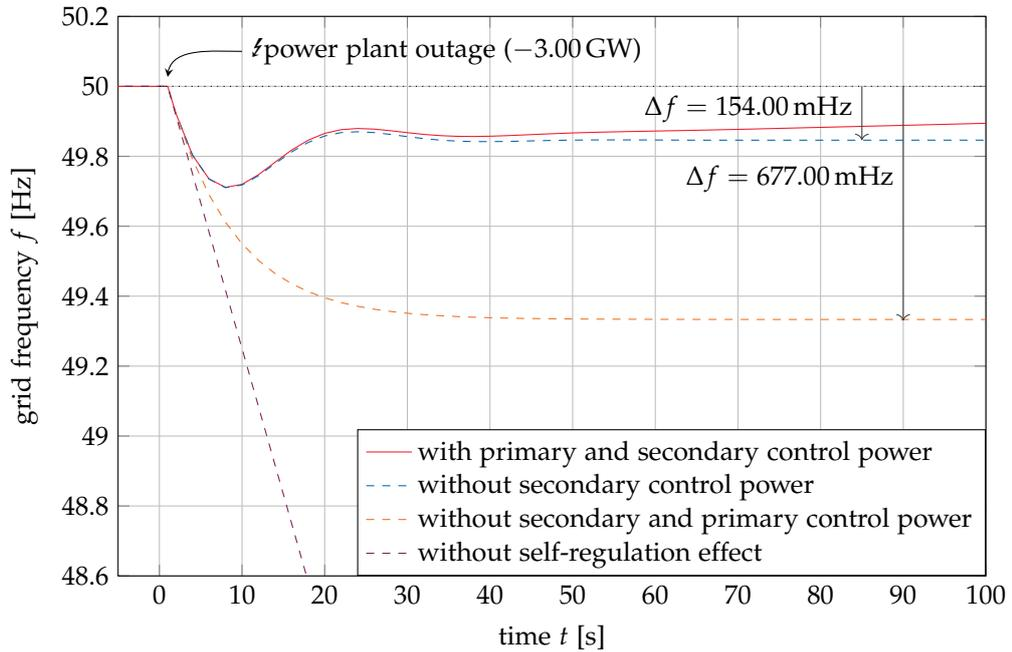
(a) Response of the grid frequency. Dashed curves show the frequency response without the named effects.
