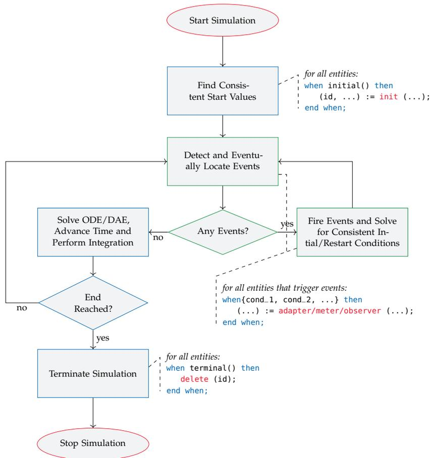
Figure 51: MOCES synchronization process and its interaction with the structure of the algorithm used to perform a simulation of a HDAE, extended from Liu [121] and Lundvall et al. [157].
