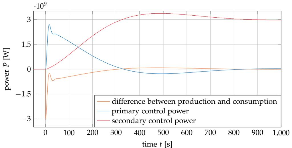
(b) Activated control power to restore the grid frequency.
