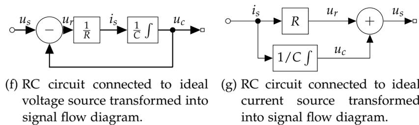
Figure 6: RC circuits in different model representations.
