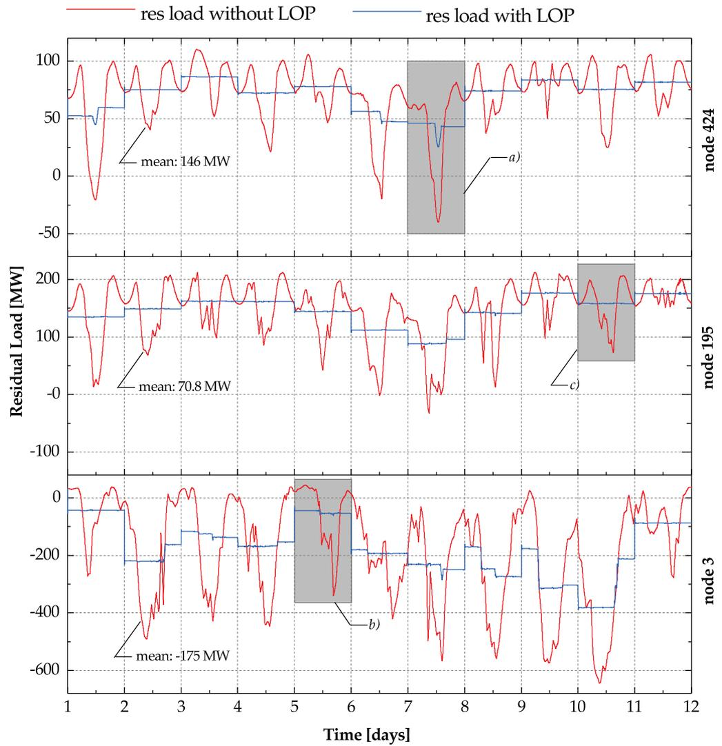
Figure 64: Exemplary temporal sequences of residual load with and without LOCAL OPTIMIZER.
