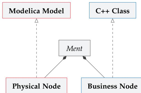
Figure 41: Basic implementation structure of a MENT.
