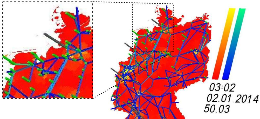
Figure 57: Visualization of simulation results in DYMOLA. Besides the line usage (right color bar) and the load density of the regions (left color bar), it shows the feed-in at the respective nodes with stacks perpendicular to the plane. The color indicates the source (green: wind, grey: conventional, yellow: PV). The numbers on the right show the time, date and grid frequency.
