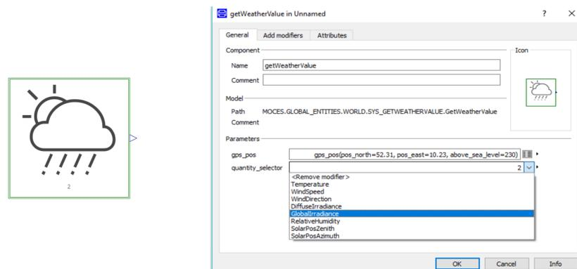
Figure 47: Model icon of `GetWeather` model (left) and its dialog showing the parameters (right).
