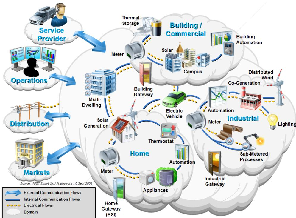
Figure 16: Customer domain of the NIST CONCEPTUAL MODEL, taken from [5].
