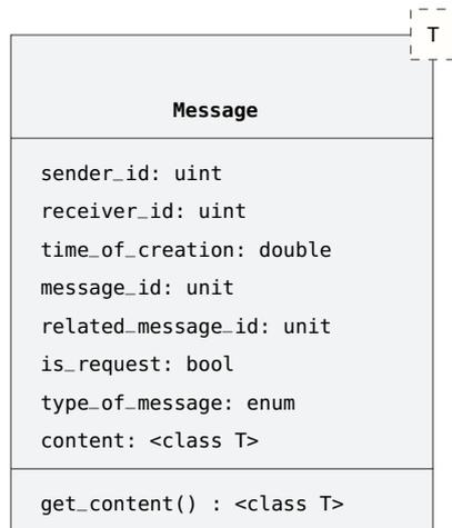
Figure 52: Class diagram of the message enabling communication between *Business Nodes*.
