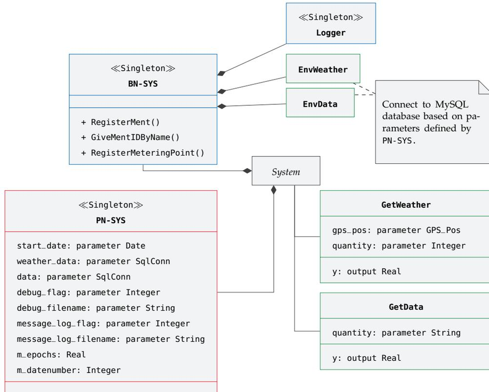
Figure 46: Simplified class diagram of the MENT System showing crucial elements.
