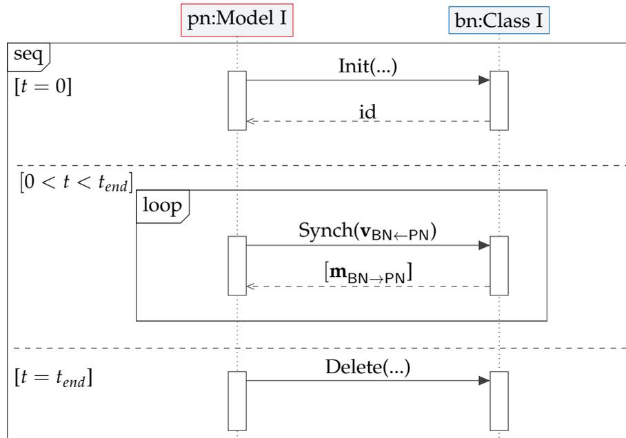
Figure 43: Fundamental interactions between *Physical Node* (pn:Model I) and *Business Node* (bn:Class I) during simulation ( $0 < t < t_{end}$ ), its initialization phase ( $t = 0$ ), and termination phase ( $t = t_{end}$ ). The notation of the variables in the simulation phase aligns with the notation introduced in Section 4.3.
