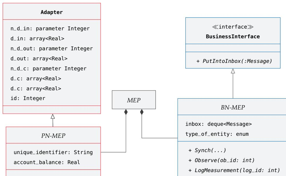
Figure 44: Simplified class diagram of the abstract base class MEP showing the most important attributes and methods.
