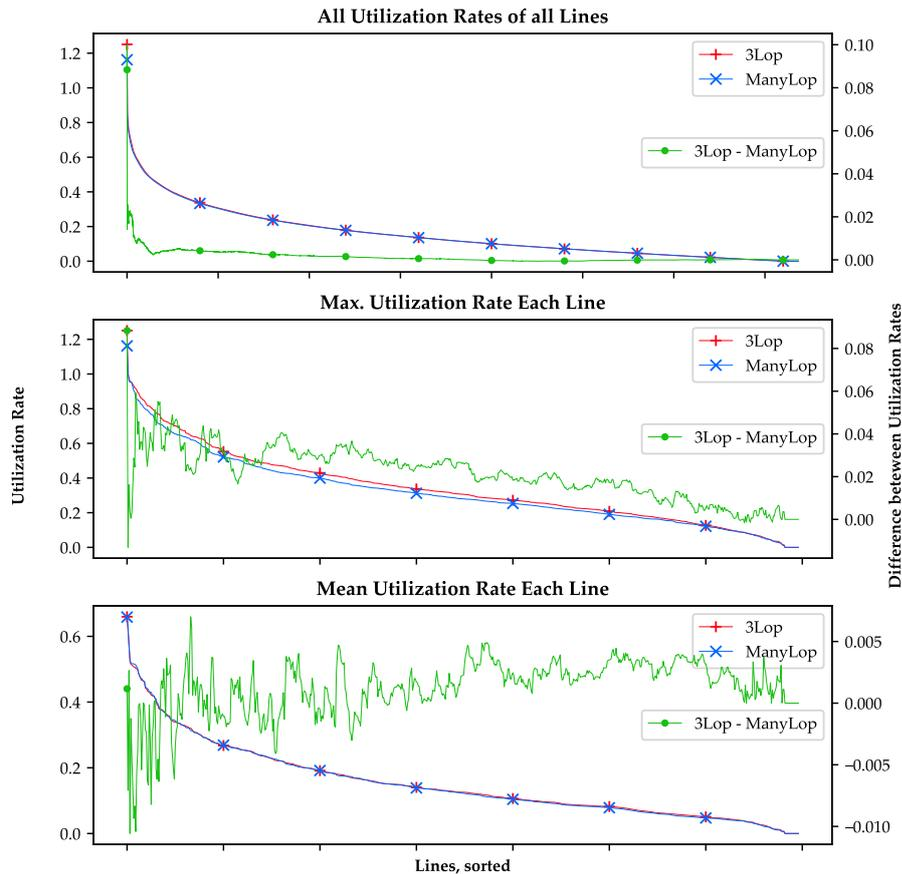
Figure 74: Details about the network load in the scenarios 3Lop and ManyLop: Utilization rate per line and scenario sorted by load. The green line shows the difference between the two scenarios. The topmost graph uses all lines and all time slices. The graph in the center uses only the time slice with the maximum load from the individual lines. The lower graph uses the average value per line.
