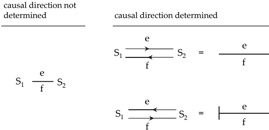
Figure 5: Notation for bond graphs, adapted from Paynter and Briggs [20].
