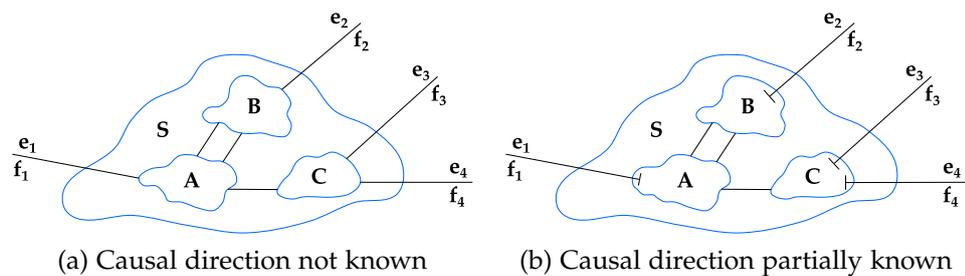
Figure 4: Abstract depiction of a system of systems connected by *energy bonds* represented by bond graphs, adapted from Paynter and Briggs [20].
