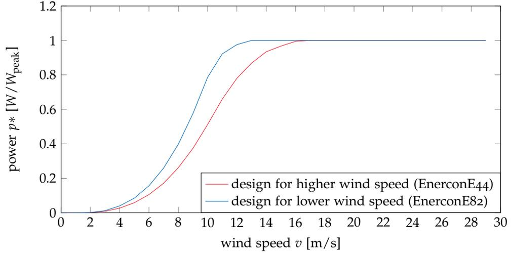
Figure 60: Typical power curves for wind power plants used in *Scenario Base Model*, data taken from [165].
