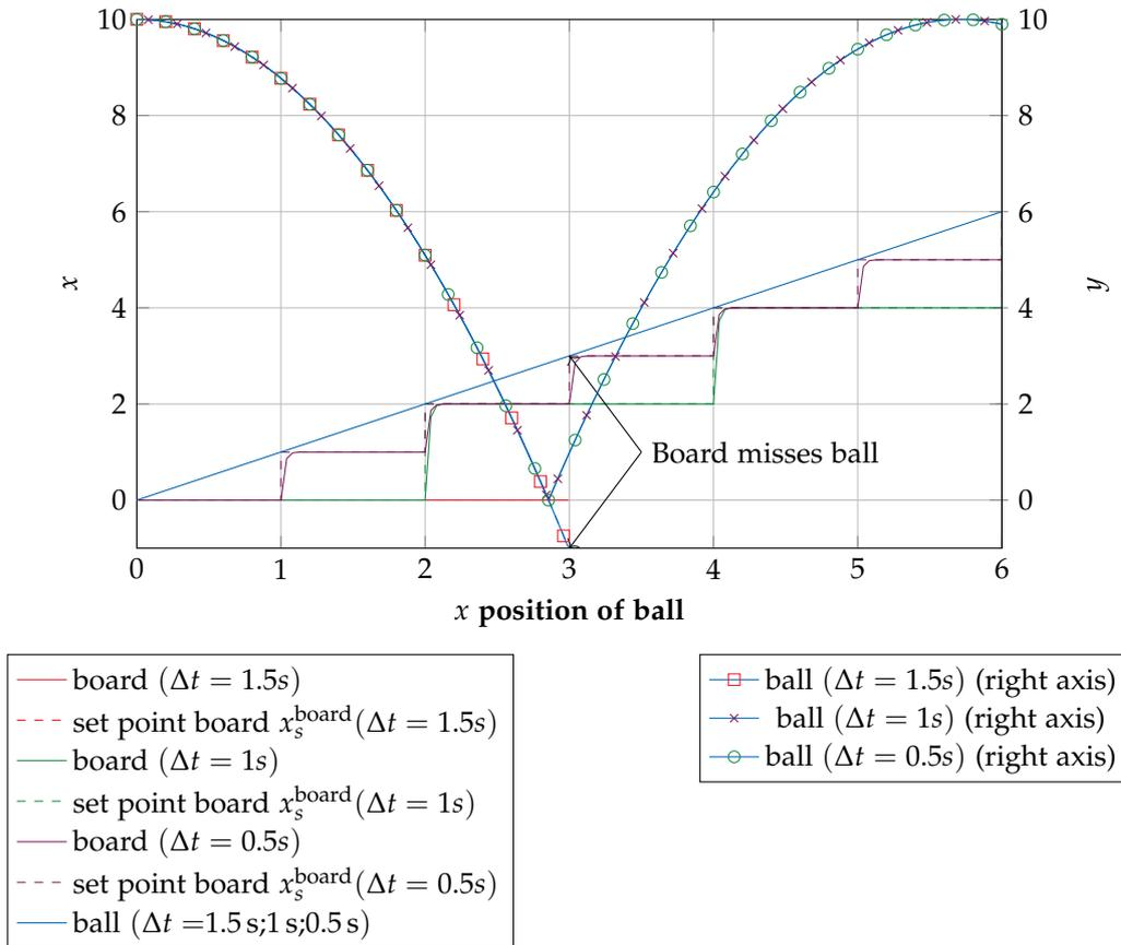
Figure 40: Behavior of board and ball for the *fixed time step scheduling* approach. Behavior is given for different values of  $\Delta t$ . If  $\Delta t$  is set to 1.5s, the board misses the ball as the gap between the board's  $x$  position and the ball's  $x$  position is not covered by the board's width, see the position marked with "Board misses ball".
