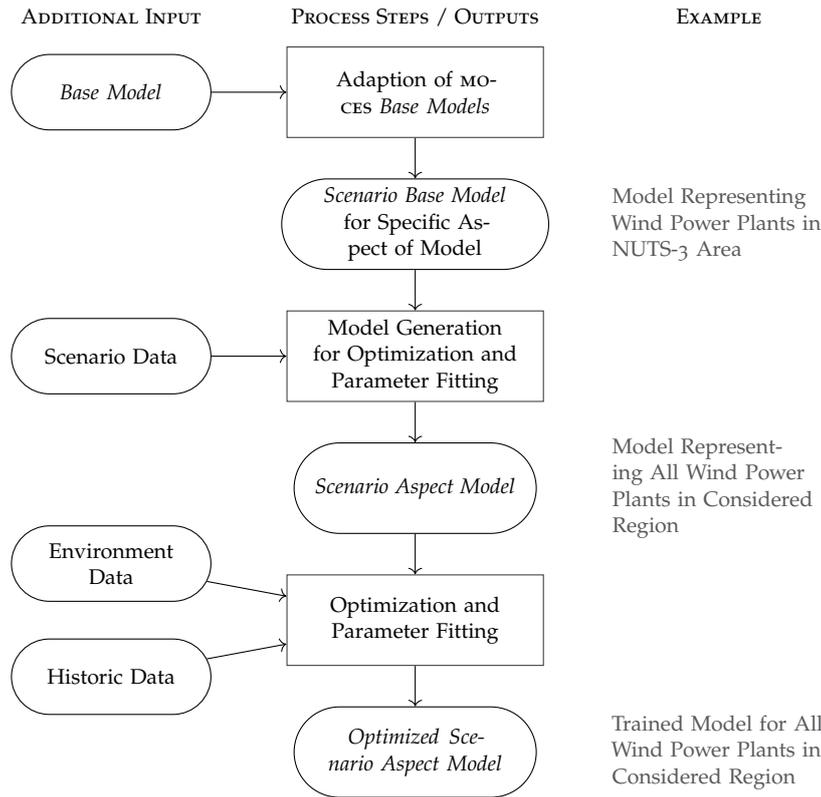
Figure 58: First phase of the modeling and simulation process in MOCES.
