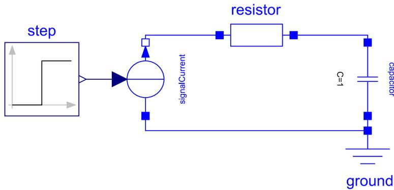
Figure 27: MODELICA diagram representing an RC circuit.
