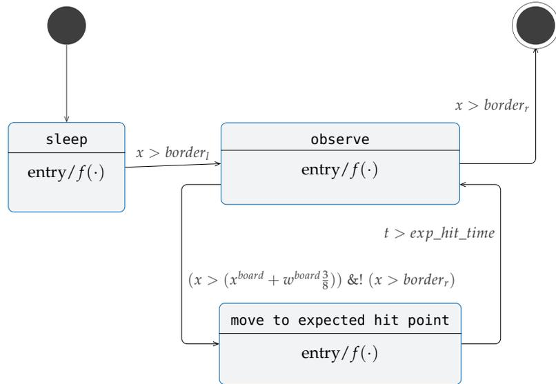
Figure 36: State machine of the *Business Node* performing actions on the linked *Physical Node* representing the board.
