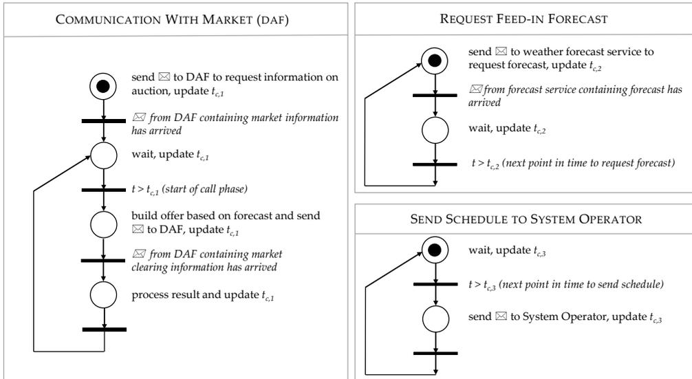
Figure 55: Exemplary behavior of the *Business Node* of a MENT describing a PV plant described by a set of Petri nets. The acronym DAF stands for ‘day ahead flex’ and is derived from the chosen model name for a day market in MOCES.
