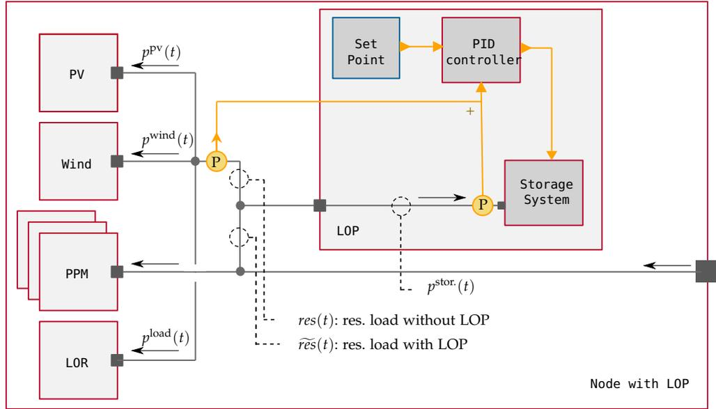
Figure 63: Structure of a node with a LOCAL OPTIMIZER entity. PPM (Power Plant Market) represents a conventional power plant assigned to the node; LOR (Load Region) models the load of the region represented by the node.
