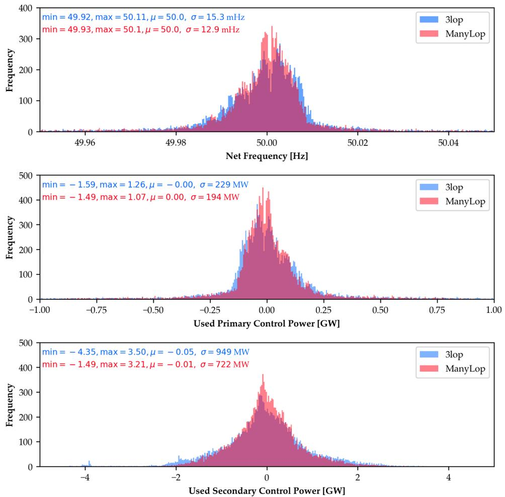
Figure 77: Histograms of grid stability metrics. To calculate the metrics, the period shown in Figure 75 without the first 24 hours was used.
