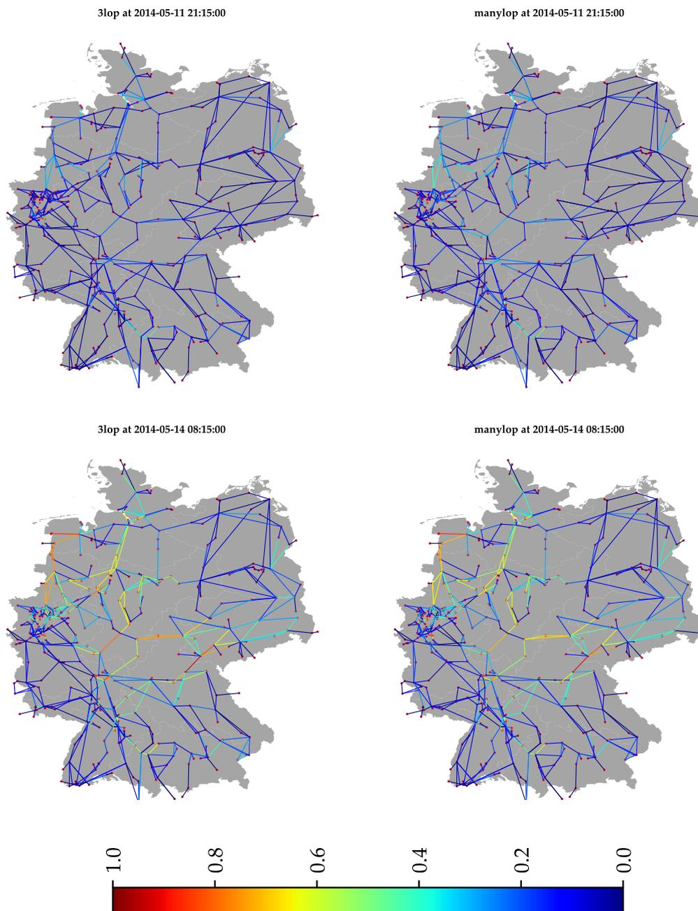
Figure 76: Network load in the different scenarios for the points in time with minimum (top) and maximum (bottom) network load. The load is given by the utilization rate of the line. See also Figures 74, 75.
