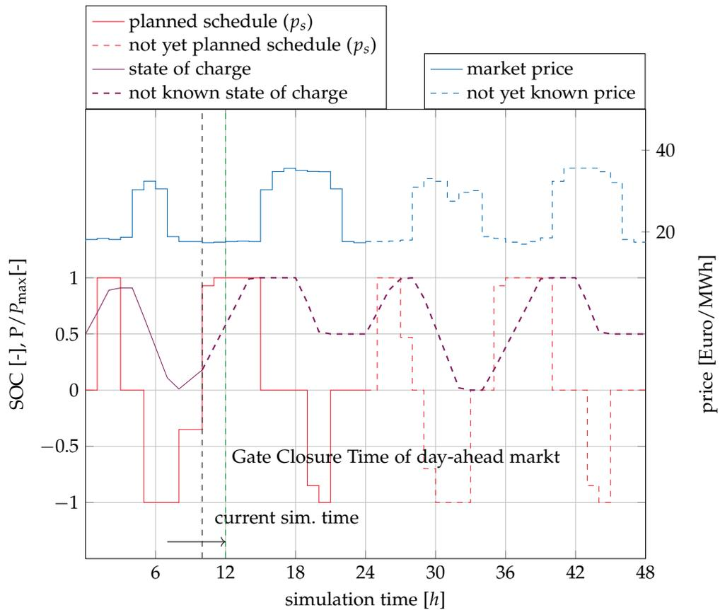
Figure 56: Visualization of the challenge of the storage system to find an optimal schedule. Dashed lines indicate, that the represented information is not known at the current simulation time that is given by the black dashed vertical line. The green vertical line indicates the GCT.
