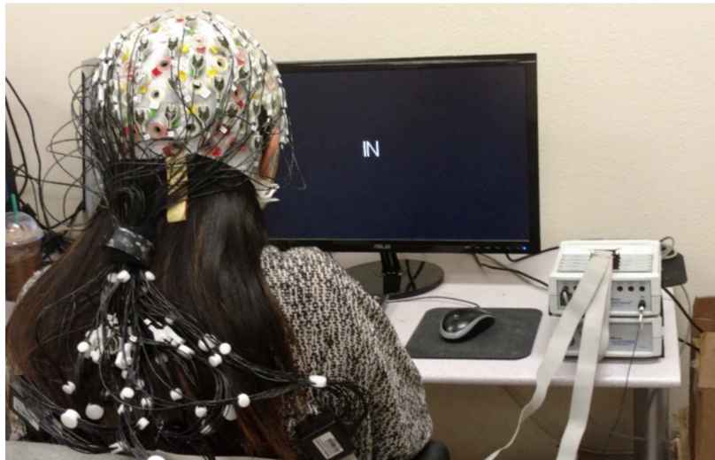
Figure 2.15: Study setup of Nguyen et al. as presented in [156]. The participant wears a stationary 64 channel headset and is seated in front of a screen for target presentation.
