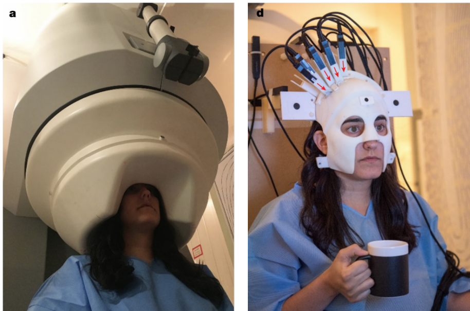
Figure 2.1: A conventional MEG device on the left and the newly developed portable solution on the right, as presented in [25]. The conventional SQUID based solution is comparably bulky like the fMRI while the new solution based on OPMs allows the user to move and e.g. hold a cup.
