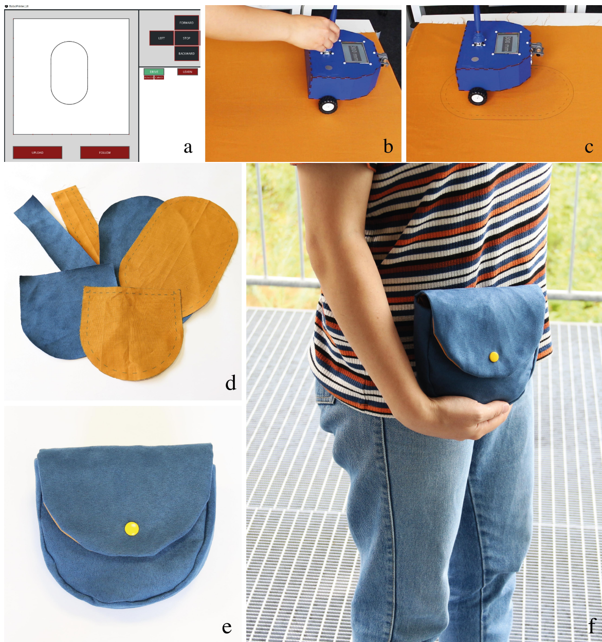
Figure 5.14 Creating sewing patterns on fabric: a) uploading the design, b) scaling the design on the fabric, c) the robot prints the pattern on the fabric, d) cutouts with sewing marks, e and f) fabricated clutch bag.
