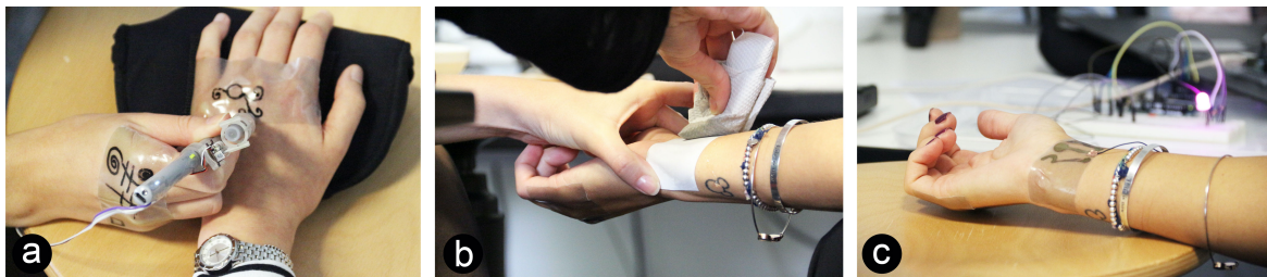
Figure 3.15 Artists during focus group exploration. Inking on each other (a), applying substrate for functional prototype interface (b), completed epidermal interface controlling an RGB LED (c).
