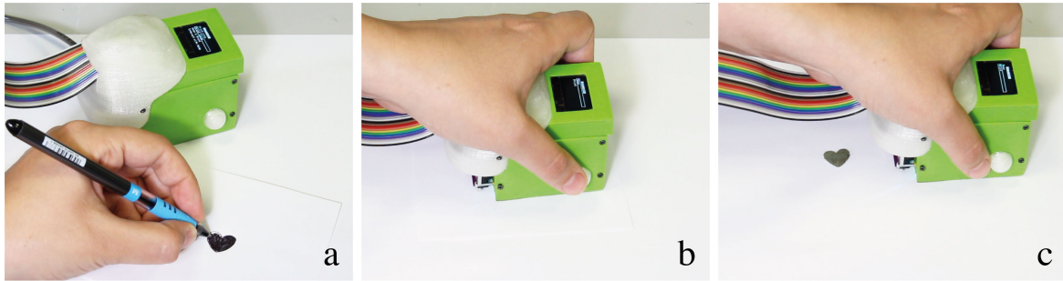
Figure 4.10 Scan & Print: a) Sketching custom design, b) scanning, c) and printing the design.
