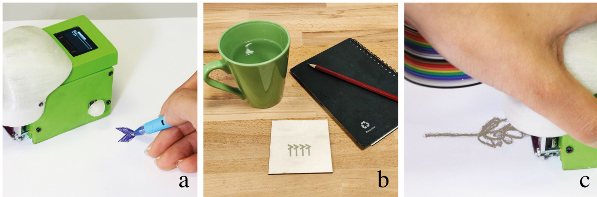
Figure 4.21 Images from user study: (a) drawing a customized electrode to scan & print, (b) Printed design based on the hand-drawn electrode. (c) free-form sketching.
