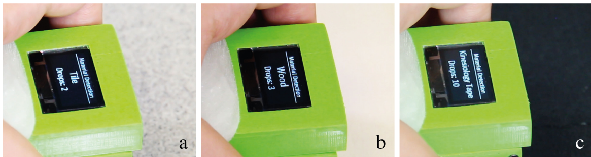
Figure 4.17 Adjusting the printing parameters to the detected materials: a) tile, b) plywood, 3) kinesiology tape.
