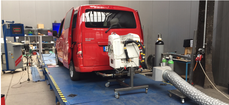
Figure 6.2: Nissan NV200 Evalia on a dynamometer
