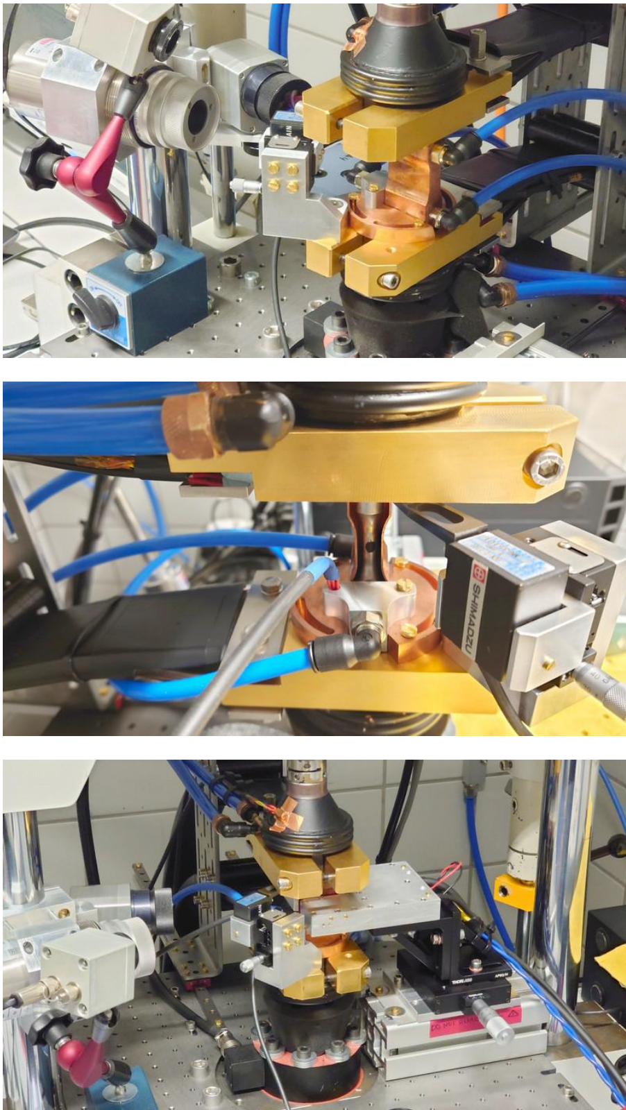
Fig. 30. Views of the fatigue specimen mounted in the servo-hydraulic thermo-mechanical setup. The specimen is covered by the water-cooled copper heat shield. The uniaxial magnetic balance is inserted over the heat shield.
