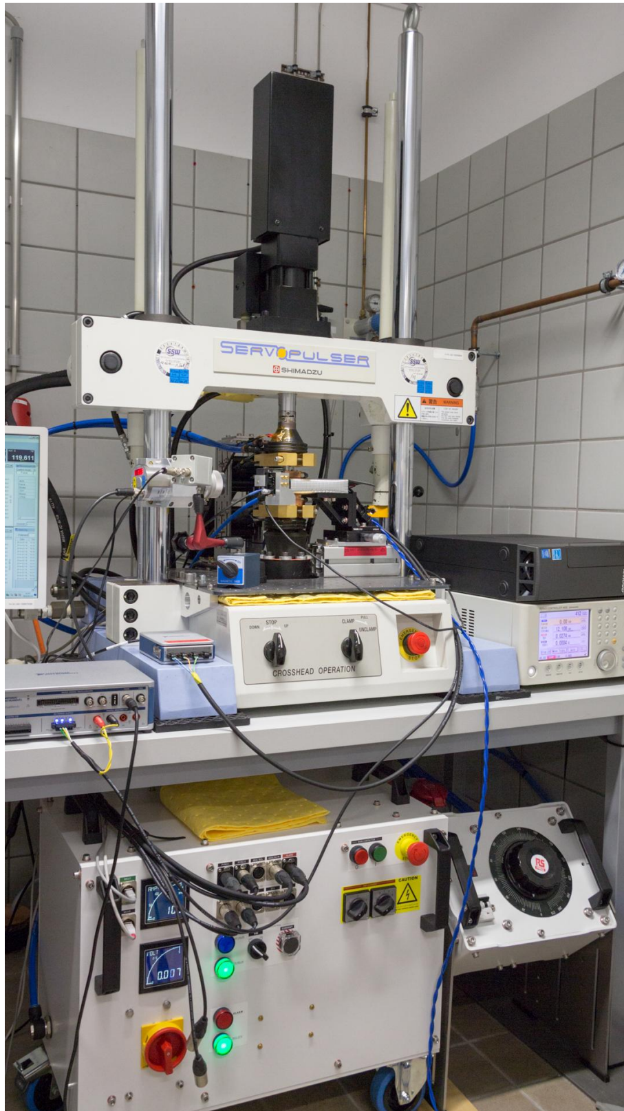
Fig. 31. A photograph of the thermo-mechanical power unit (at the bottom) and Shimadzu Servopulser servo-hydraulic fatigue testing machine with mounted uniaxial magnetic balance.
