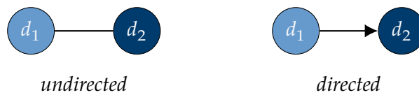
Figure 2.3: Directed and undirected developer networks: (left) vertices d_1 and d_2 are connected by an undirected edge; (right) vertices d_1 and d_2 are connected by a directed edge, that is, d_1 is the initiator of the interaction (e.g., d_1 changes a file that d_2 has already changed beforehand).
