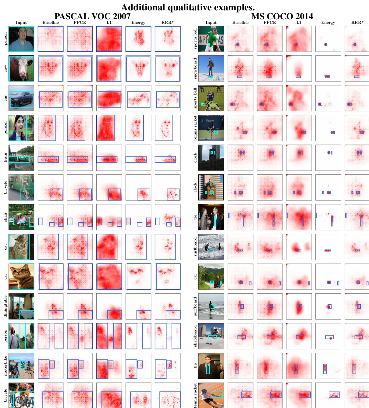
Figure D.3: Qualitative examples from the VOC (left) and COCO (right) datasets. In particular, here we just show additional examples for the B-cos models with input attributions, as this configuration exhibits the most detail. We show results for such models trained with different losses ( columns ) for multiple images ( rows ).
