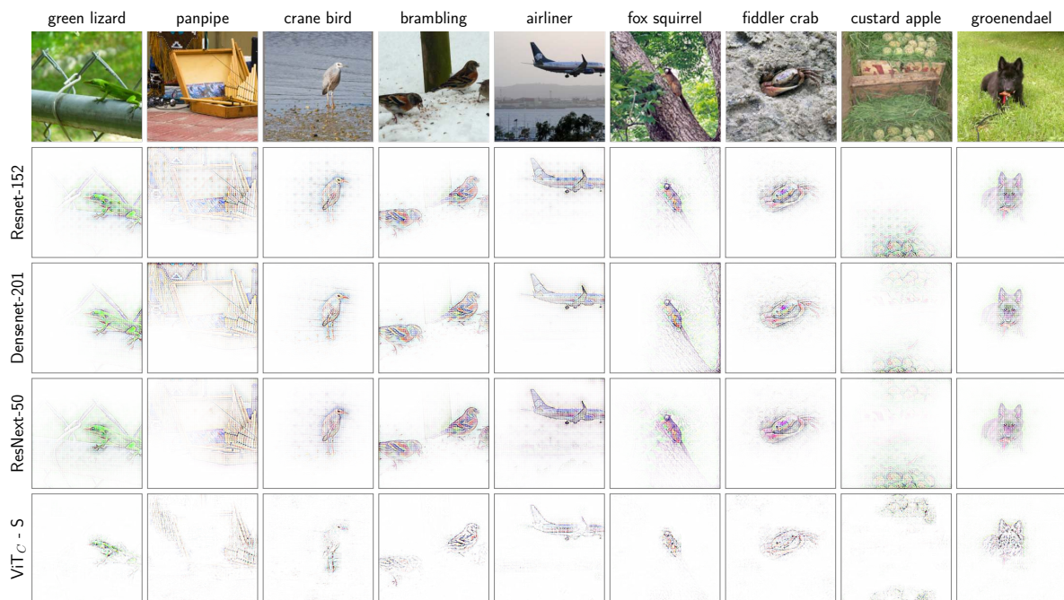
Figure C.2: Additional model explanations based on \mathbf{W}(\mathbf{x}) for various B-cos architectures, see also Figure C.3. While the explanations are generally consistent between models, architecture-specific details can be observed. E.g., ResNet-based architectures exhibit a grid-pattern in the explanations, and we find that the ViT models generally produce sparser explanations.
