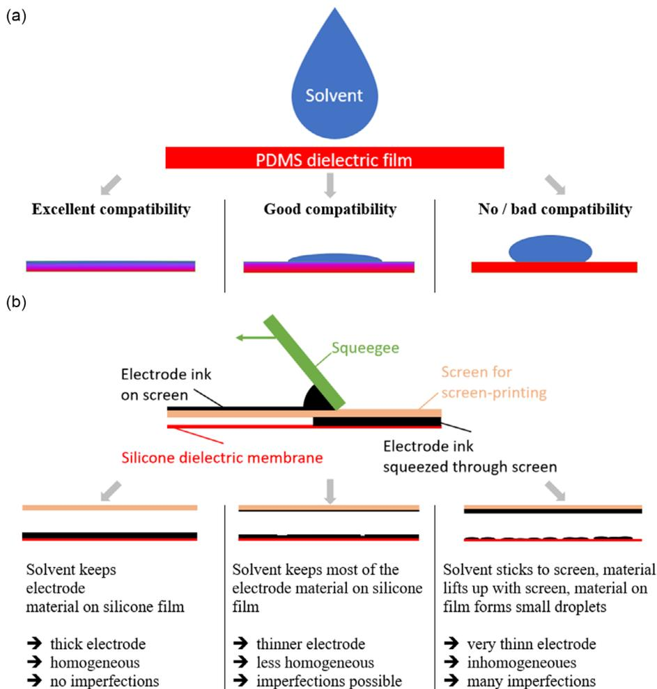
**Figure 7.** a) Influence of compatibility between solvent and PDMS dielectric film when pure solvent is put on the film, and b) when using the solvent in the printing material for screen-printing. It is schematically shown how an excellent, a good and a bad compatibility between solvent/printing material and dielectric film influences the behavior while screen-printing.
