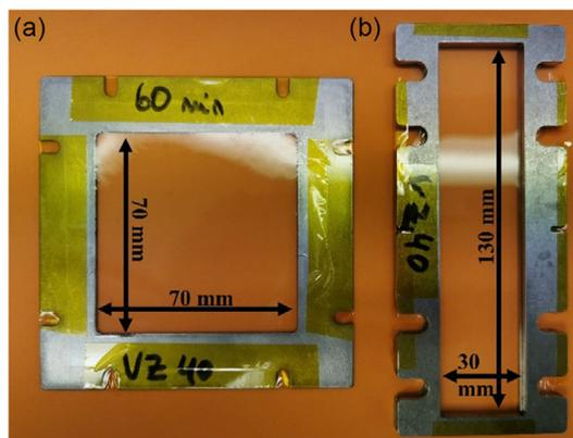
**Figure 1.** a) Sample geometries for Elastosil 2030 PDMS film treated with pure solvent for optical measurements, and b) breakdown tests.
