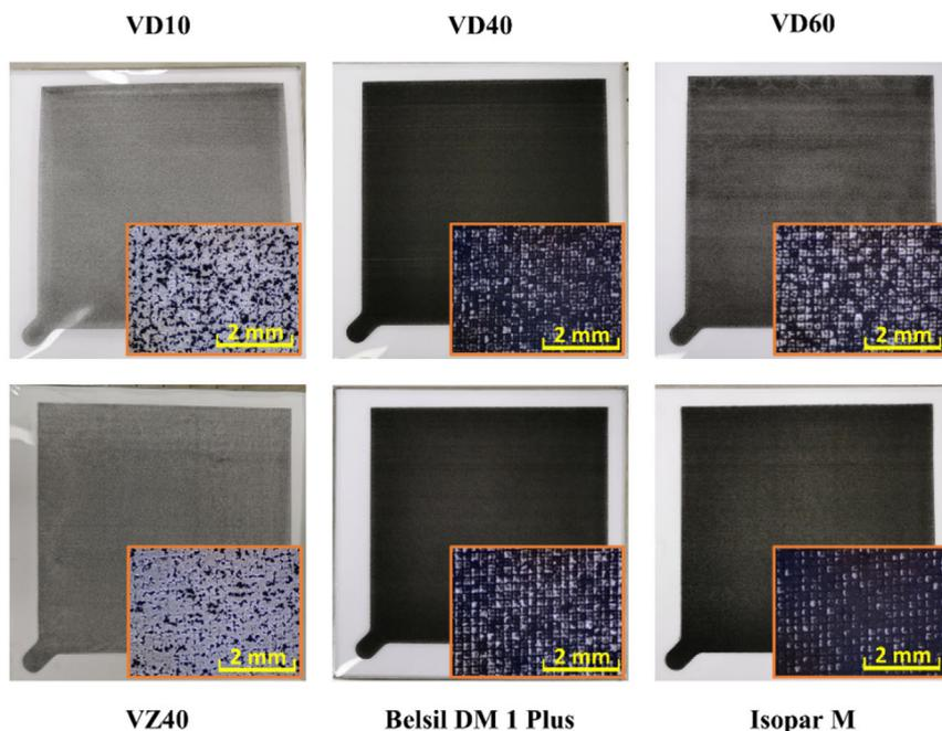
**Figure 6.** Photos of screen-printed electrodes and enlarged microscopic images of the electrodes printed with different solvents.
