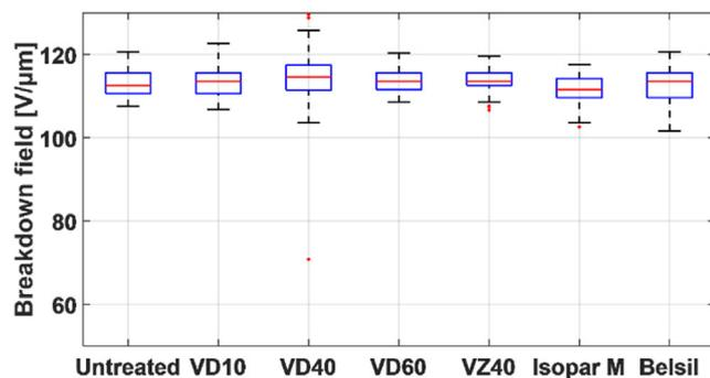
**Figure 5.** Breakdown fields of the untreated silicone membrane and of the solvent-treated silicone membranes.
