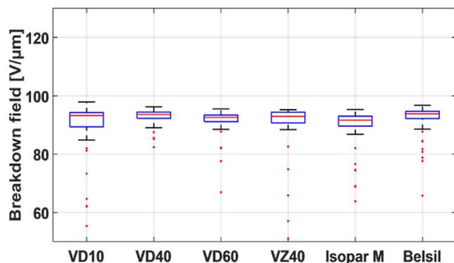
**Figure 8.** Breakdown fields of the silicone membrane after applying screen-printed CB-electrodes manufactured with different solvents.
