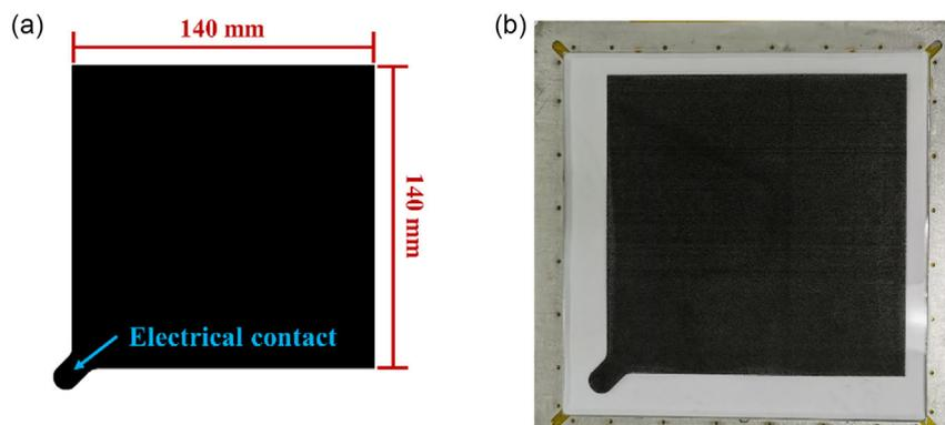
**Figure 2.** a) Schematic electrode geometry: a square with the edge length of 140 mm completed with a contact region in the lower-left corner; b) image of an actual screen-printed electrode with this design.
