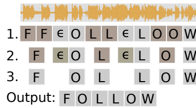
Figure 2.7: CTC algorithms steps, After the initial sequence prediction (1), repeated characters are merged, followed by the removal of the blank token.
