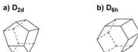
Figure 7: Structures of T_{12}^R , a) less symmetrical structure ( D_{2d} ), b) higher symmetrical structure ( D_{6h} ). Each corner represents one silicon atom, and each edge represents one oxygen atom. Adapted from reference [149].
