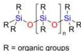
Figure 5: Exemplary representation of a linear siloxane.
