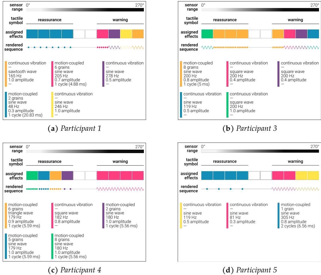
Figure C.1: Tactile symbols designed by the participants to communicate reassurance and warning. These symbols were experienced on knobs.
