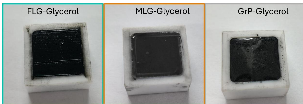
Figure S5.8: Electrofluids prepared with different 2D carbonaceous fillers in glycerol. From left to right FLG, MLG, and GrP as filler particles.
