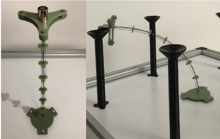
Figure 6: The SMA Continuum Robot, showcasing bio-inspired motion using SMA wires.
