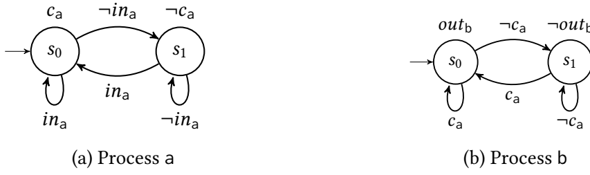
Figure 1.2 An implementation of a bit transmission distributed systems with 2 processes. Process a receives an input bit from the environment on in_a and transfers its value to process b via the communication variable c_a . Process b reacts to c_a by setting out_b equivalent to c_a .
