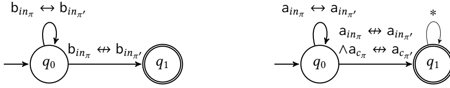
(a) The prefix distinguishability automaton. (b) The prefix information-flow automaton.
