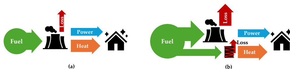
Figure 1. Conceptual comparison of efficiencies for (a) combined and (b) separate heat and power generation.
